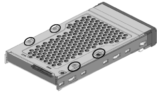
Figure 2-21-2. Installing 3.5-inch SAS/SATA Drive
